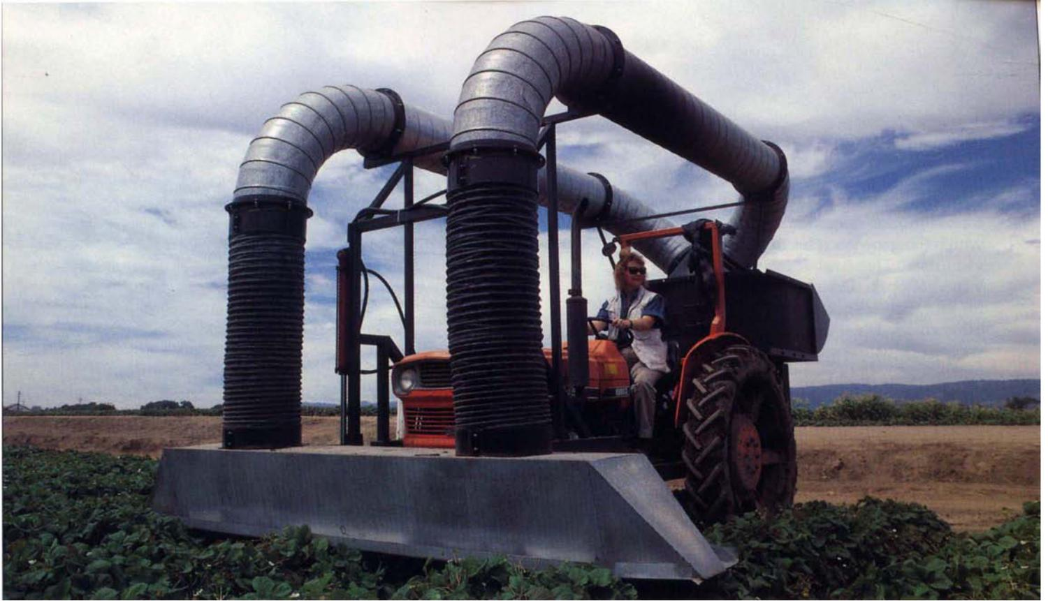
**This three-bed vacuum machine reduced Lygus bug abundance and strawberry damage to a greater degree than the smaller machines.**
