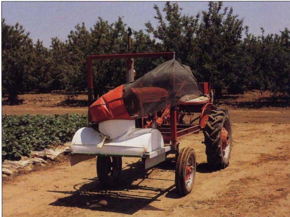
**This single-bed vacuum machine, made by a grower-cooperator, uses an apple sprayer fan. It was modified in 1990 to vacuum two beds.**
