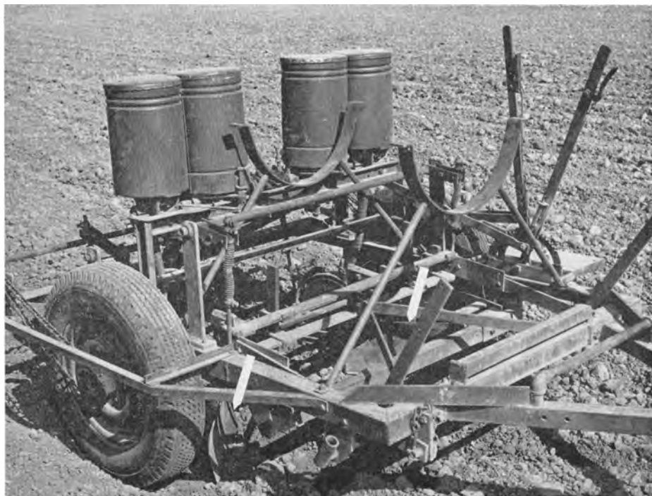
Experimental two-row Range Seeder. Machine was built light and compact to facilitate transportation. Note scraper blades arrows to the front and inside of the wheels, and the double disc furrow openers. Center hoppers are for fertilizer. Outer hoppers are for seed. Cradle is to support drum used with spray equipment.
