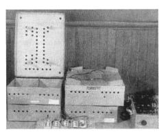
Equipment used in determining the effect of temperature inside chick and poult boxes. Wires lead to thermocouples inside boxes.
