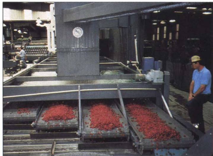
A hydrocooler is used to rapidly cool cherries before they are placed into boxes.
