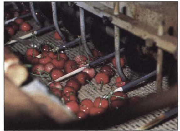
In the most widely used type of cluster cutter, fruit clusters are carried on a moving belt through banks of closely spaced rotating saws. Plastic tines lift the stems of clusters off the belt and guide them into the vertically mounted saw blades.
