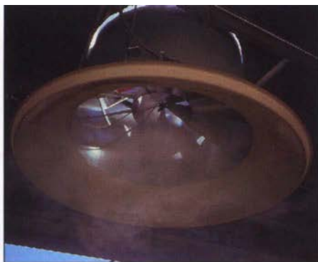
Korral Kool, which is used in a partially enclosed area, combines a fine mist with air movement (detail above) and costs about $400 per cow.
