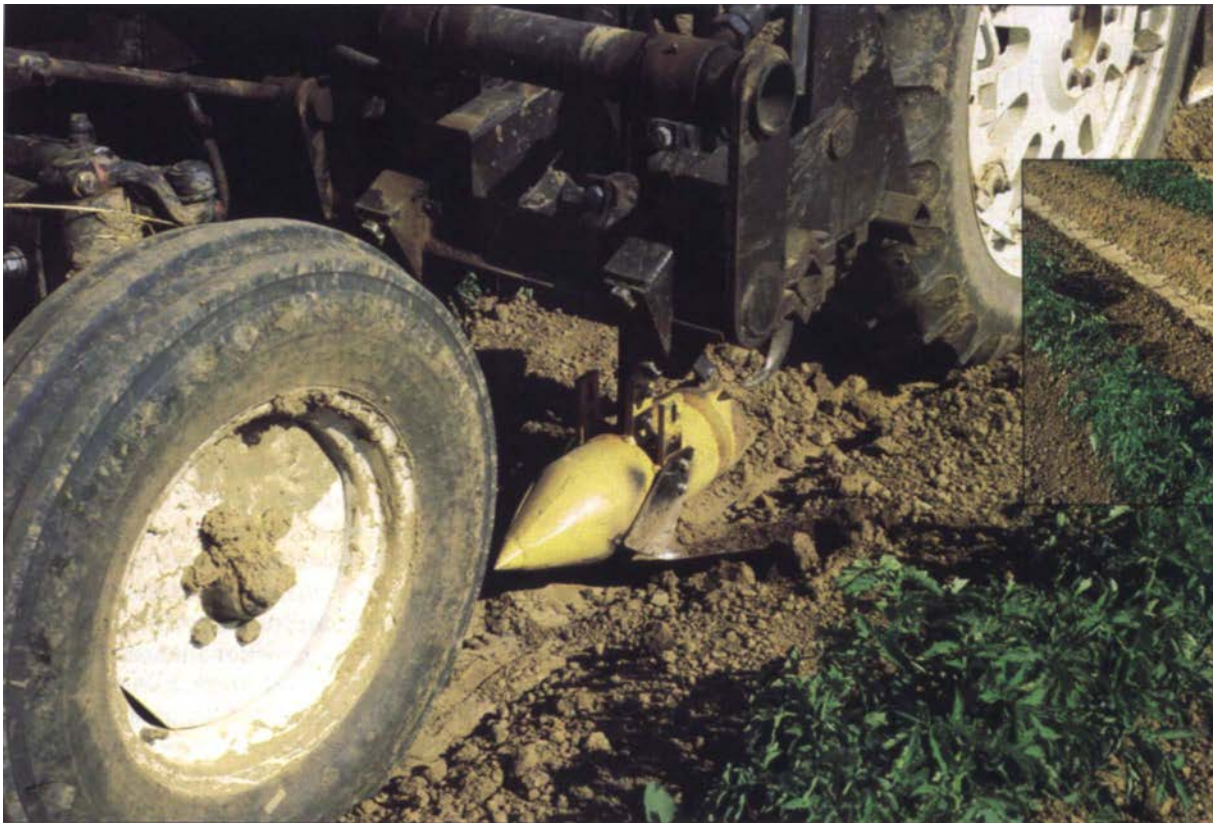
A torpedo-shaped, winged crust-breaking device crushes through the crust on the soil surface in a tomato field. Inset, soil crusting impedes water penetration.
