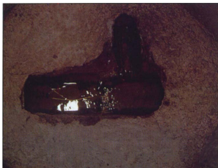
Scientists blocked the drains at junctions, like the one shown above, to observe the effect on salinity and water-table depth in heavy soils in the Imperial Valley.
