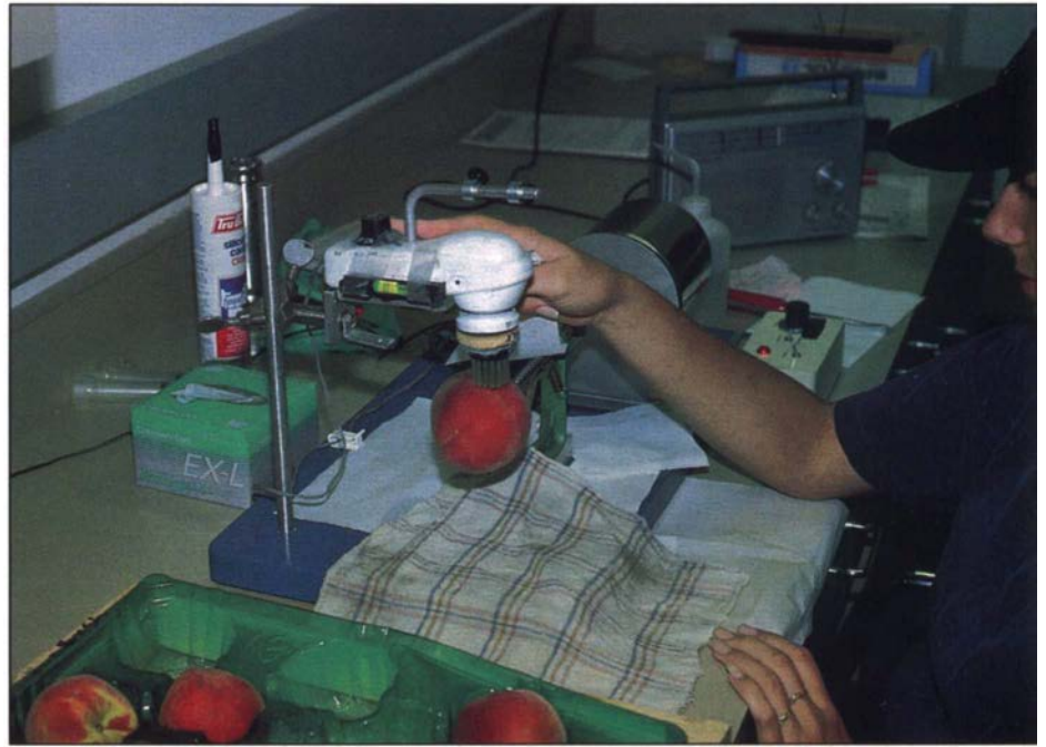
Some of the fruit were abraded to study the role of injury in inking. The fruit were abraded with a rotatable automatic toothbrush and a fruit holder.
