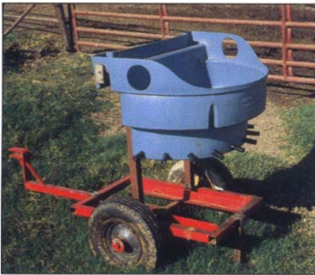
This portable feeder can accommodate 10 calves and can be easily towed by a 4-wheel all-terrain vehicle (ATV). Any other needed supplies can be taken out to the paddock in the same trip.
