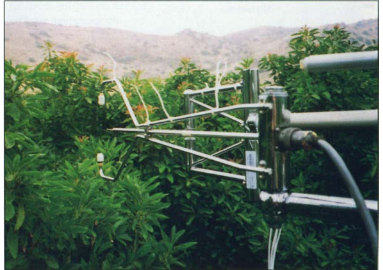
Eddy covariance measurements over avocados near Camarillo.
