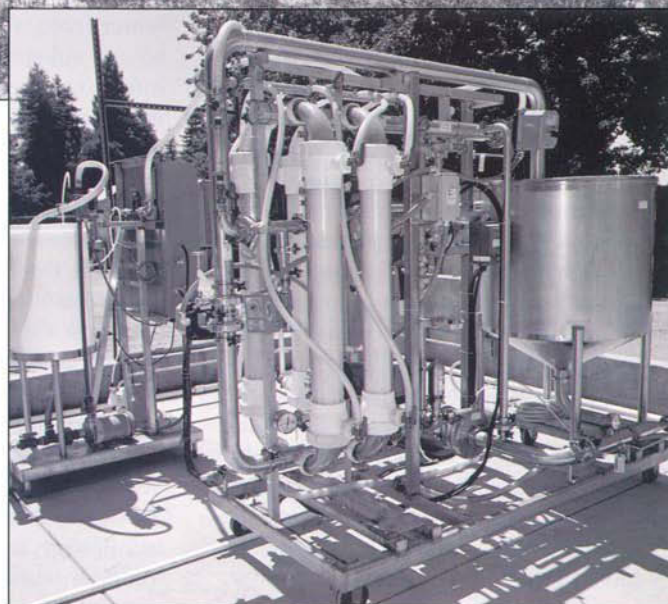
Above, A large, conventional water-treatment plant utilizes coagulation, flocculation and filtration. Right, A small, packaged ultrafiltration-membrane-system pilot plant is being tested at UC Davis.
