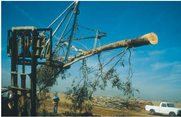
Finally, trees were weighed with a forklift and crane scale. The authors found that river red gum trees did best when irrigated with at least 4 acre-feet of water per year and at about 900 trees per acre; fertilizer did not have an effect.
