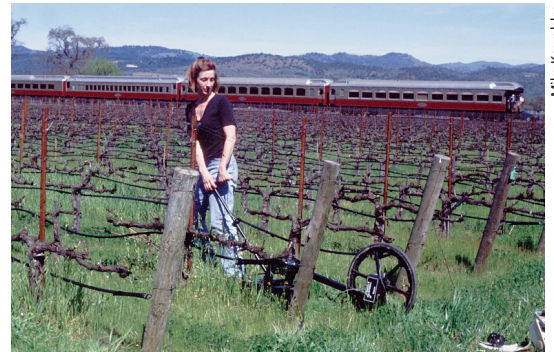
UC Davis hydrogeophysicist Susan Hubbard uses GPR to map soil moisture at the Robert Mondavi Winery.
