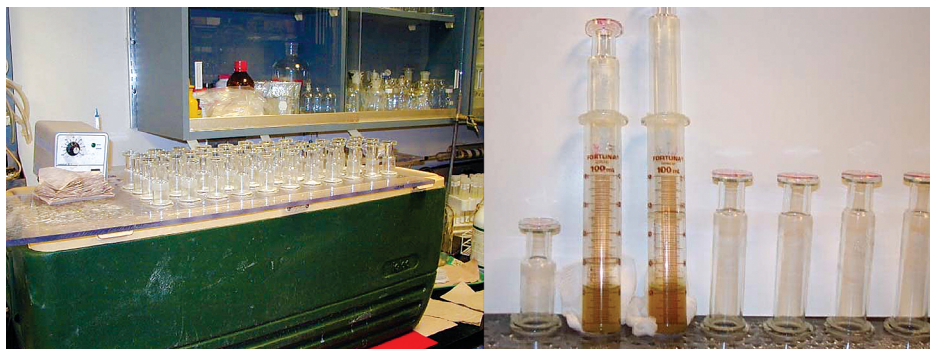
Left, dozens of syringes containing feed samples can be incubated at the same time during a single 24-hour incubation run. Right, gas production is measured by reading the scale on the side of the syringe.
