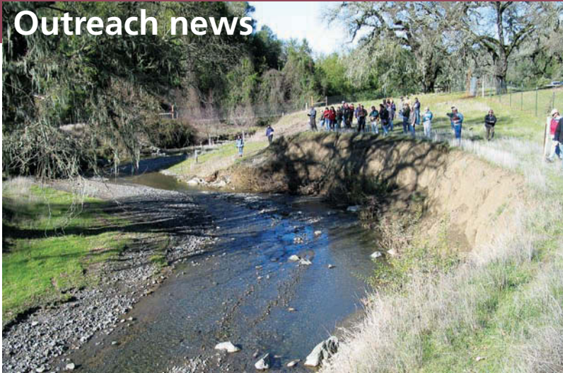
Water-quality short course participants evaluate a sediment source site (bank-cutting) along Parson's Creek using the Sediment Inventory Method, at the UC Hopland Research and Extension Center in Mendocino County.
