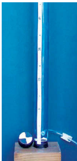
Typical transparency tube used to make water-clarity measurements. Water is released from the outlet valve until the black-white target at the bottom of the tube becomes visible.
