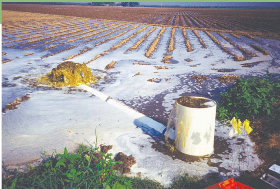
Researchers measured water discharge into the field by placing plastic hydrants over alfalfa valves with a Doppler flow meter attached.
