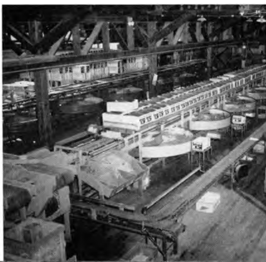
Three types of packing equipment for pears and apples. Left, packing bins used in many fruit packing houses. Center, one model of packing tubs. Right, the modern revival of an older method—packing directly from conveyor belts.
