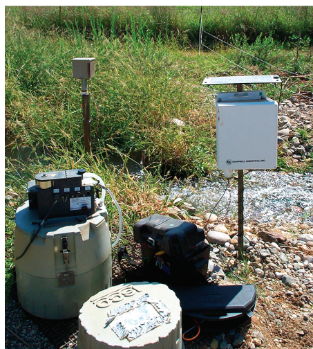
Top left, channelized runoff from the pasture was collected in a small basin. Above, V-weirs were fitted with, left, autosamplers to monitor E. coli concentrations.
