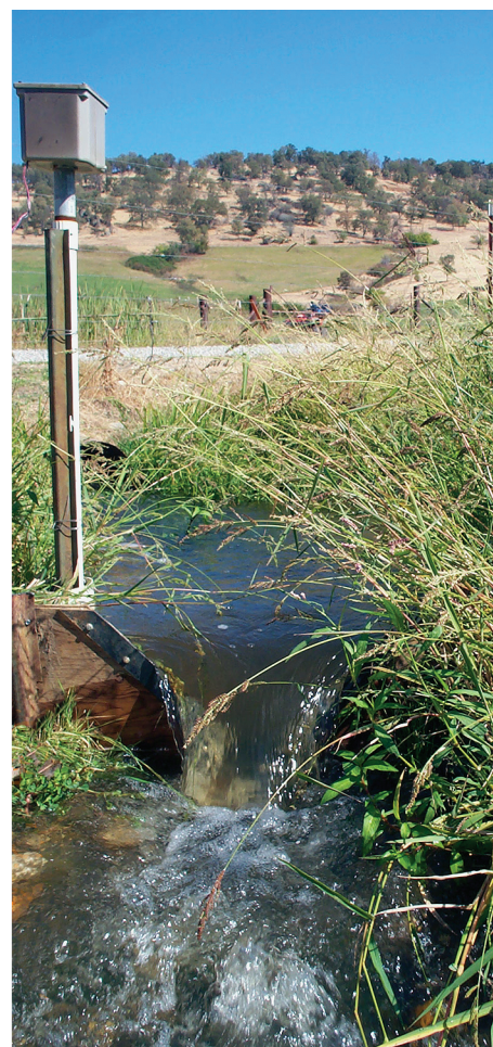
Top left, channelized runoff from the pasture was collected in a small basin. Above, V-weirs were fitted with, left, autosamplers to monitor E. coli concentrations.
