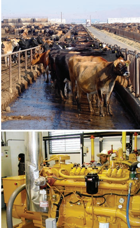
Top , manure from dairy cattle is used as a feedstock for anaerobic digestion to produce biogas (primarily methane and carbon dioxide), which, above , generates electricity at the Castelanelli Dairy in Lodi.
