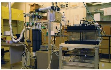
Rats were exposed to airborne particulate matter via an aerosol concentrator (VACES) in inhalation chambers.
