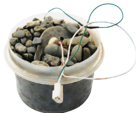
The wetting-front sensor consists of a plastic container surrounded by a gravel and sand jacket.
