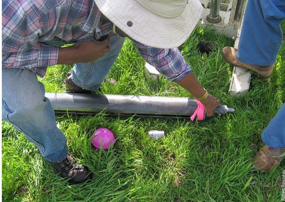
To characterize soil quality, researchers took soil samples and measured soil pH, bulk density and moisture. Above, soil core and GPS located marker ball at Dixon Ridge Farms.
