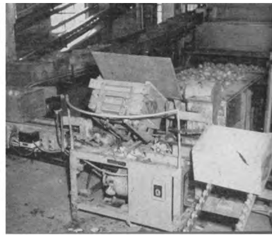
Single-box dumping machine. Field lugs are fed by conveyor from the left to a dumping table, which tips and empties the box, then delivers empty box to empty lug conveyor, right.
