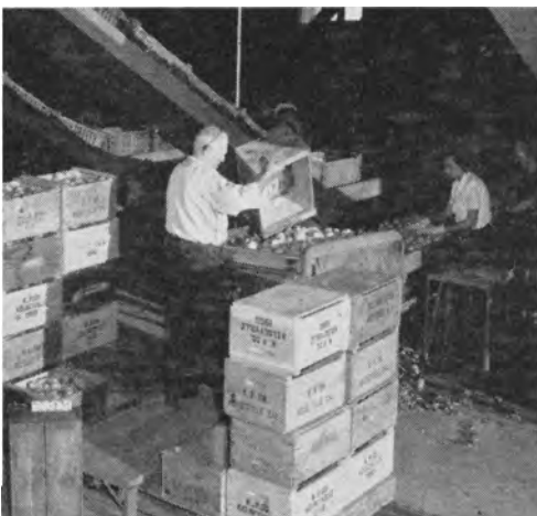
Hand dumping without conveyor aids. Lugs are supplied to the dumper on pallets—full lugs on the dumper's left and empty lugs on the right.
