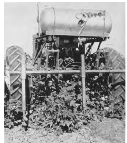
Rear view of high clearance cultivator with 24-inch sweeps.
