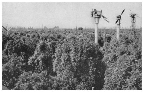
The four wind machines tested in 1953. The 93 hp machine reported is between the two with large propellers whose tests are not completed. The other 72 hp machines are not in view. The fixed helicopter machine is visible above the trees at the extreme left. Three of the eight masts for measuring overhead temperatures and velocities are also visible.
