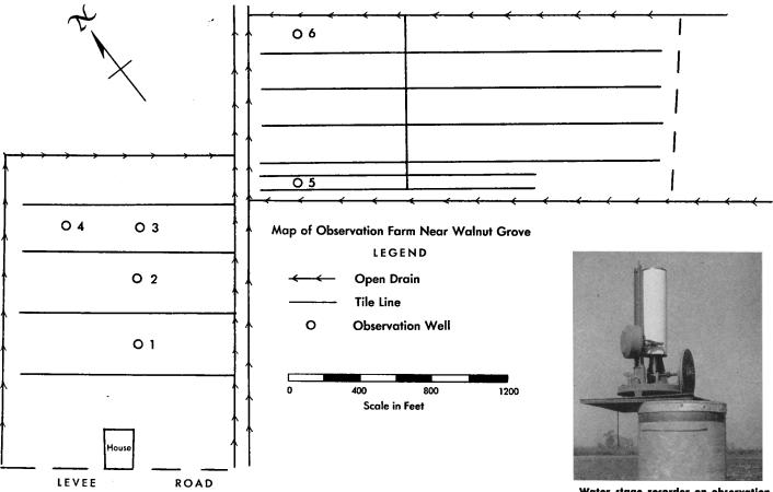
Water stage recorder on observation farm, well No. 1. Replacement of the fringe moisture is not instantaneous but depends on the speed with which water moves through the soil—its permeability.
