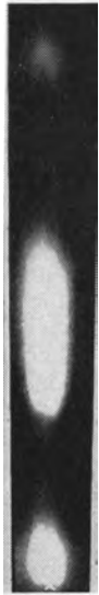
Radioautograph of a chromatogram of labeled technical demeton. The lower spot is demeton, the middle spot is isodemeton, and the top spot is impurities.
