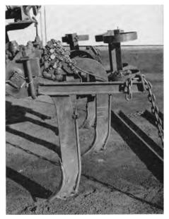
Close-up showing detail of injection chisel.
