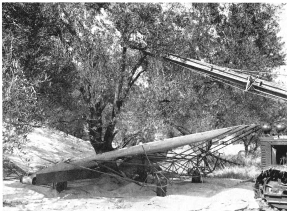
Above: Position of attachment of shaker arm to tree and placement of catching frame. Below: Type of mechanical shaker used in mechanical olive harvesting tests.
