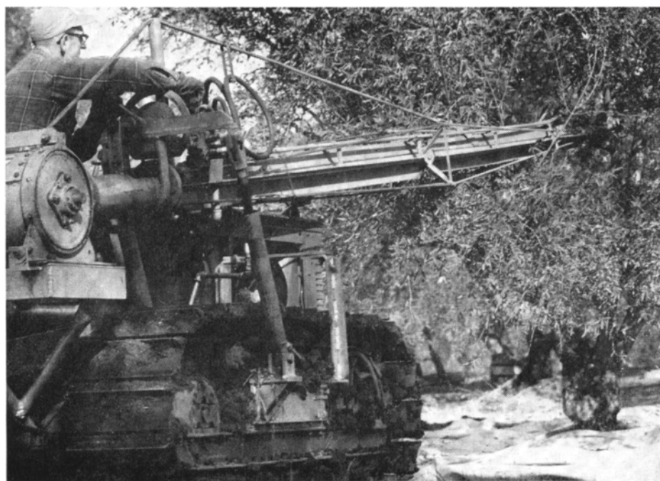
Above: Position of attachment of shaker arm to tree and placement of catching frame. Below: Type of mechanical shaker used in mechanical olive harvesting tests.
