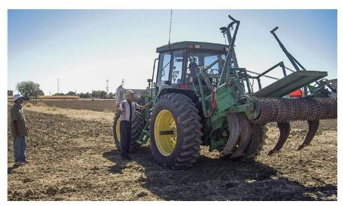
Trial results suggest that GPS-controlled spot fumigation has the potential to reduce fumigant use. Above, testing the fumigant applicator at UC Davis.
