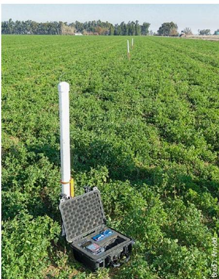
When a sensor (white pole) detects water arrival, a wireless signal is sent to the central module (black box), which generates a text message alert to the irrigator.
