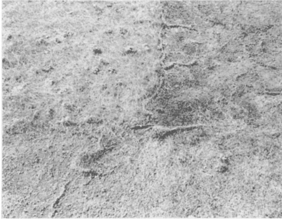
FIG. 6. Small terraces of soil and fine mulch washed from a bare plot during a storm of high intensity on October 18, 1953. Movement of materials was not obvious on the plots with a mulch cover.
