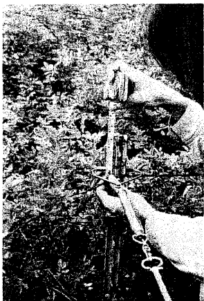
Figure 18. — Measuring from the top of the stake to the tension spring handle.
