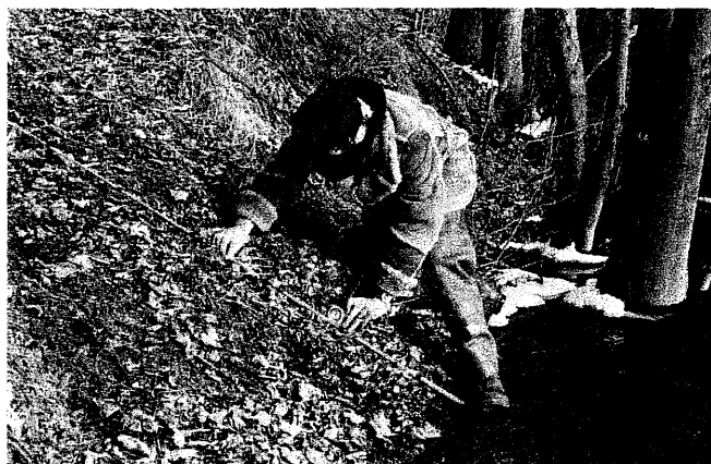
Figure 10. — Using a clinometer to measure a bank angle of 145^\circ .
