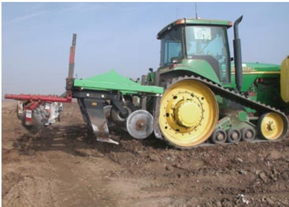
Figure 1. Terratill bent leg subsoiling shank implement (Bigham Brothers, Lubbock, Texas) used to loosen soil profile following crop harvest.
