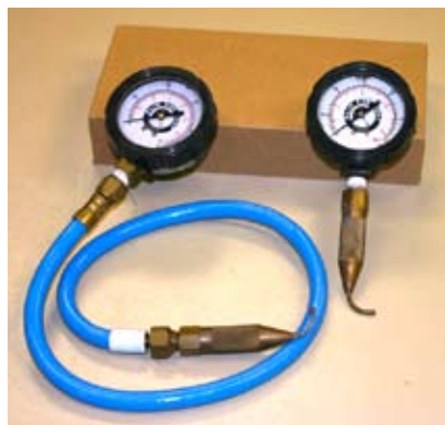
Figure 3. Pressure gauge fitted with a pitot tube to measure sprinkler nozzle pressure. Photo: Lawrence J. Schwankl.
