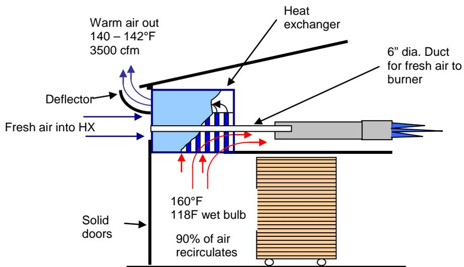
Figure 3. Schematic of passive heat exchanger installed in a transite prune dryer
