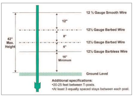
Figure 26. Specifications for a four-strand wildlife-friendly fence. Modification to existing fences can be made by replacing the bottom wire with a smooth wire that is at least 12 inches off the ground.(Adapted from Heffelfinger et al. 2006). Smooth wire (12 1/2 gauge) is recommended for the top wire (barbed wire may be required for protecting riparian or wetland areas).
