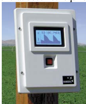
AM 400 logger can accept 6 Watermarks and Temp sensor. $389
