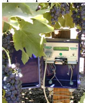
8 channel Irrrometer logger for Watermark sensors. $389
