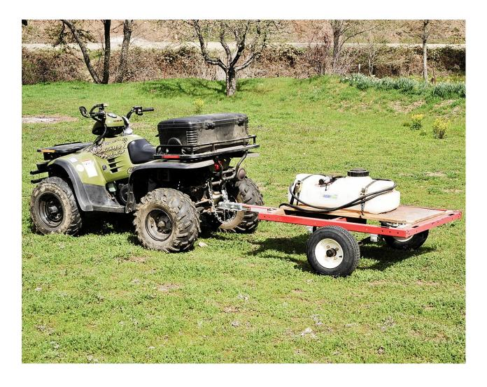
15 gallon 12v electric tank sprayer on a mini-trailer
