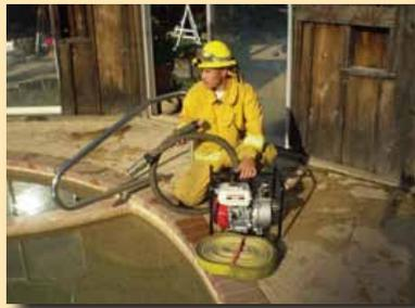
backwards out of the hose. This is very helpful in initially establishing flow through the pump and maintaining flow if you need to stop and re-start the pump. The discharge should be compatible with your fire department's fittings.
