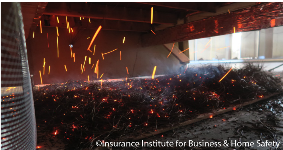
Embers passing through gaps between deck boards can ignite fine fuels that can accumulate under the deck, providing further evidence for the need to remove combustible materials from under the deck.
