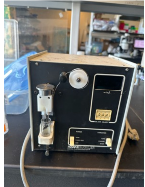
Chloride concentration is recorded with a chloridometer
