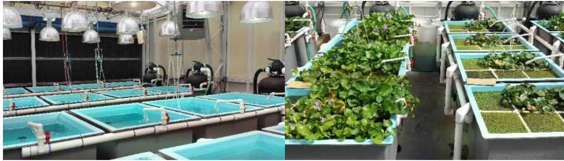
Figure 1. (Left) Experimental setup of four rows of tanks in a USDA Aquatic Weed Research Lab greenhouse. Each row is temperature-controlled at a preset temperature, with four tanks per row. (Right) Four weeks into one experiment, growth is quite apparently different between the row set at 25C (left) and the row set at 15C (right).
