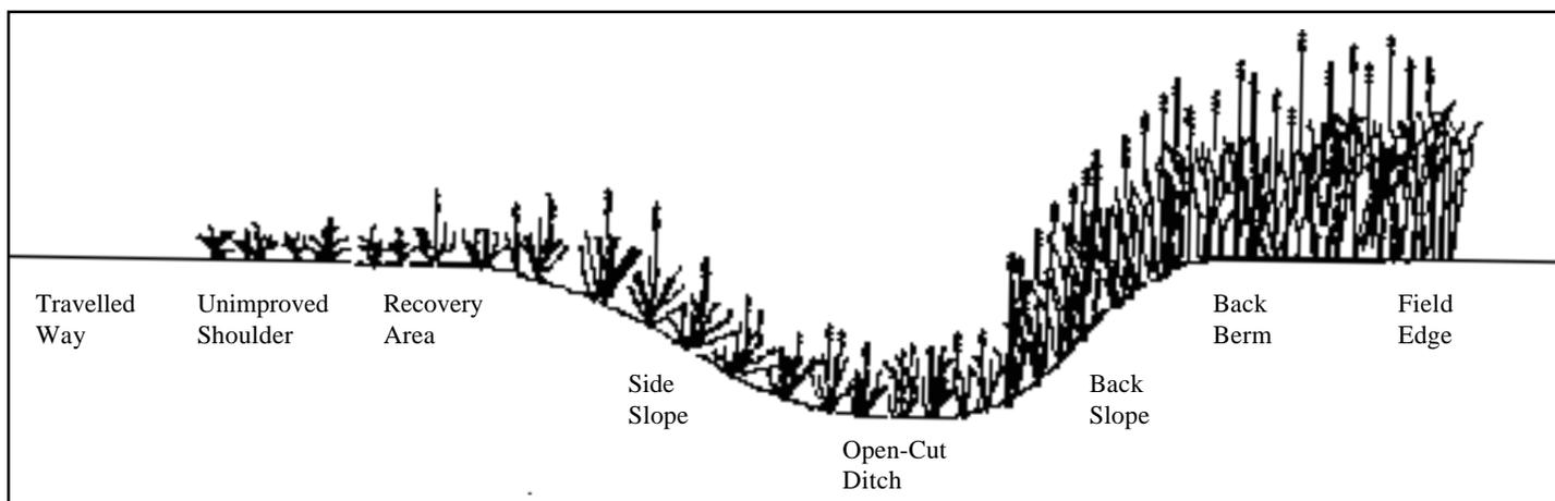
**Figure 2.** Schematic diagram of roadside topographic zones.
