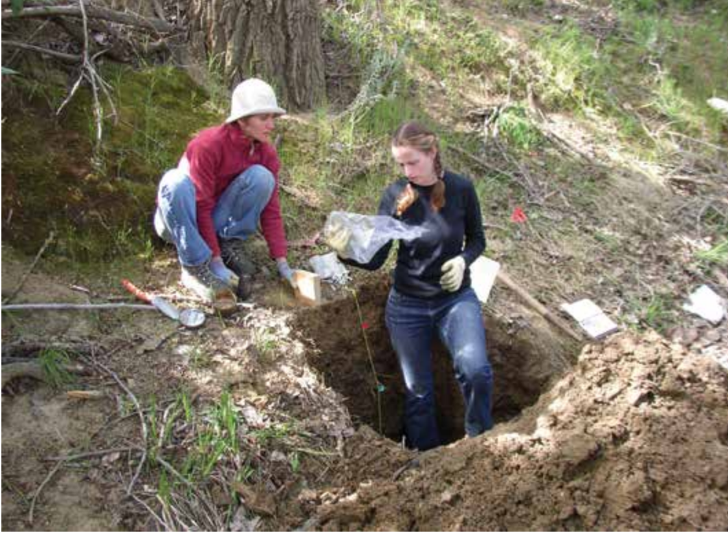
FIGURE 6. Soil pit description and sampling along the floodplain of a rangeland riparian corridor.
