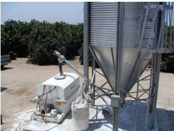
Plate 5. Gypsum injection machine attached to large silo for automatically adding bulk solution grade gypsum.
