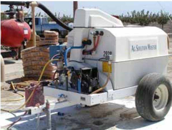
Plate 4. Mobile gypsum solutionizer machine with horizontal mixing bar for injecting gypsum slurry into drip system.
