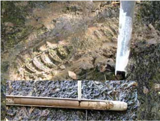
Plate 3. Surface sealing of Milham sandy clay loam in flood almonds due to low salinity, sodic well water. Penetration only to 7 inch depth after 32 hours (bottom). Surface remains saturated 8 hours after end of set.
