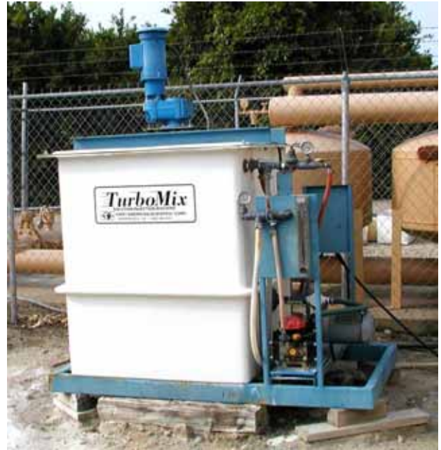
Plate 6. Batch mixer with vertical mixing bar. Suitable for dissolving some fertilizers for injection as well as solution-grade gypsum.
