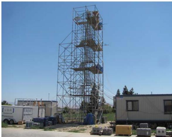
The tower on which was located numerous sampling lines, weather sensors and some analytical instruments.
