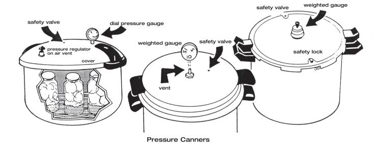
A pressure canner is a specially made heavy pot that has a lid that can be closed steam-tight. It must have a rack in the bottom, a tight-fitting cover, exhaust vent (or petcock), safety valve and an accurate pressure gauge. The pressure gauge may be a weighted gauge that fits over the vent or a dial gauge on which a needle indicates the pressure inside the canner. Newer canners may also have an extra cover lock as an added safety feature.
