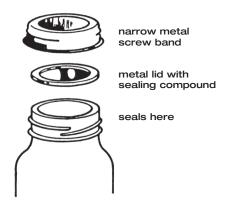
Jar lids need to be prepared for use ahead of filling time. Read the manufacturer's instructions on preparing and attaching the lids. With two-piece metal canning lids, the flat lid should be used only once for sealing new products, but the ring bands can be reused as long as they are in good condition. Ring bands should be free of rust and
