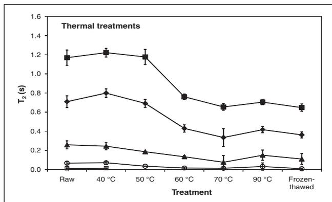
Figure 4— $T_2$  relaxation of the different components obtained by SplMod analysis (component 1 [■], component 2 [◆], component 3 [▲], component 4 [○], component 5 [□]) of raw, thermally treated (40, 50, 60, 70, and 90 °C), and frozen-thawed onions.
