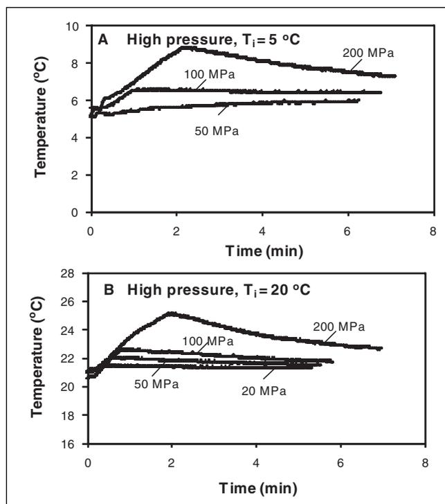
Figure 1—Temperature profile of high pressure experiments at  $T_i = 5$  °C (A) and at  $T_i = 20$  °C (B).
