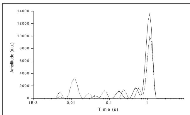
Figure 5—Example of the distributions of  $T_2$  relaxation obtained by CONTIN analysis of a 50 °C before Gd-DTPA infiltration (black line) and after Gd-DTPA infiltration (dotted line).
