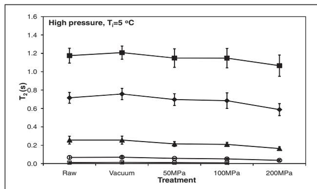
**Figure 7**— $T_2$  relaxation of the different components obtained by SplMod analysis (component 1 [■], component 2 [◆], component 3 [▲], component 4 [○], component 5 [□]) of raw, vacuum-packed, and high pressure at  $T_i = 5\text{ }^\circ\text{C}$  treated onions.
