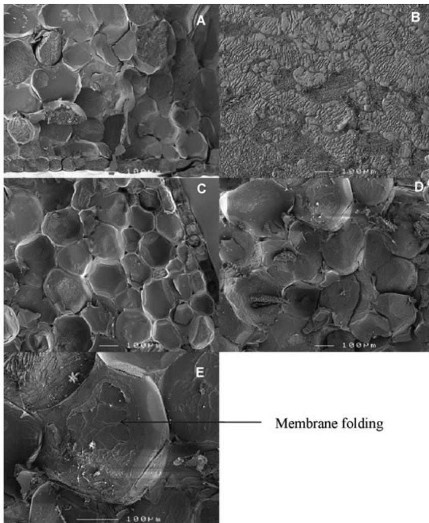
Figure 3—Cryo-SEM of onion cells. Raw tissue (A), frozen-thawed (B), high pressure at  $T_i = 5\text{ }^\circ\text{C}$  (C), high pressure at  $T_i = 20\text{ }^\circ\text{C}$  (D,E).
