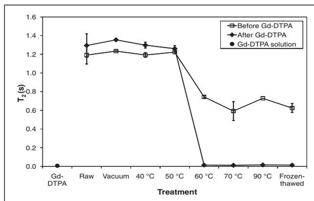
Figure 6— $T_2$  relaxation of Gd-DTPA solution and that of the average main component of raw, vacuum-packed, thermal (40, 50, 60, 70, and 90 °C) and freeze-thaw treated onions before and after Gd-DTPA infiltration obtained by SplMod analysis.
